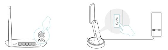
2. Within 2 minutes, press and hold the WPS button on the adapter until WPS Tool opens in the lower right corner of your computer.
